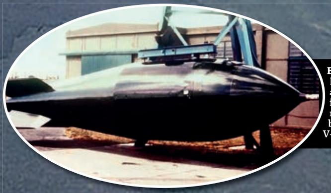
**BLUE DANUBE:** Britain's first atomic bomb. The fins extended after release allowing it to be accommodated in V-bomber bomb bays
